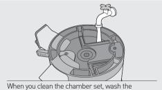
When you clean the chamber set, wash the residue inside and bottom of the chamber under running water.
