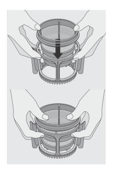
Assemble the squeezing screw into [STEP1].
