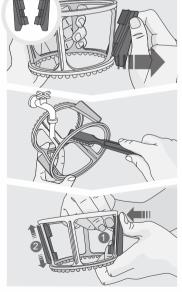
Remove the silicone brush from the spinning brush holder.
