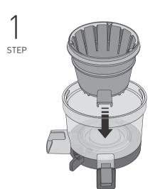
Assemble the chamber and ice cream strainer. Place the ice cream outlet align with juice outlet.
