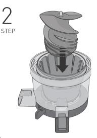
Press the squeezing screw into the assembled parts from [STEP 1] until the screw fits perfectly.
