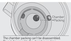
The chamber packing can't be disassembled. Do not disassemble the chamber packing. If you try to disassemble the chamber packing, it might be damaged.
