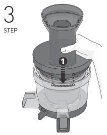
After putting the hopper on the chamber, turn it clockwise until it is locked completely.
