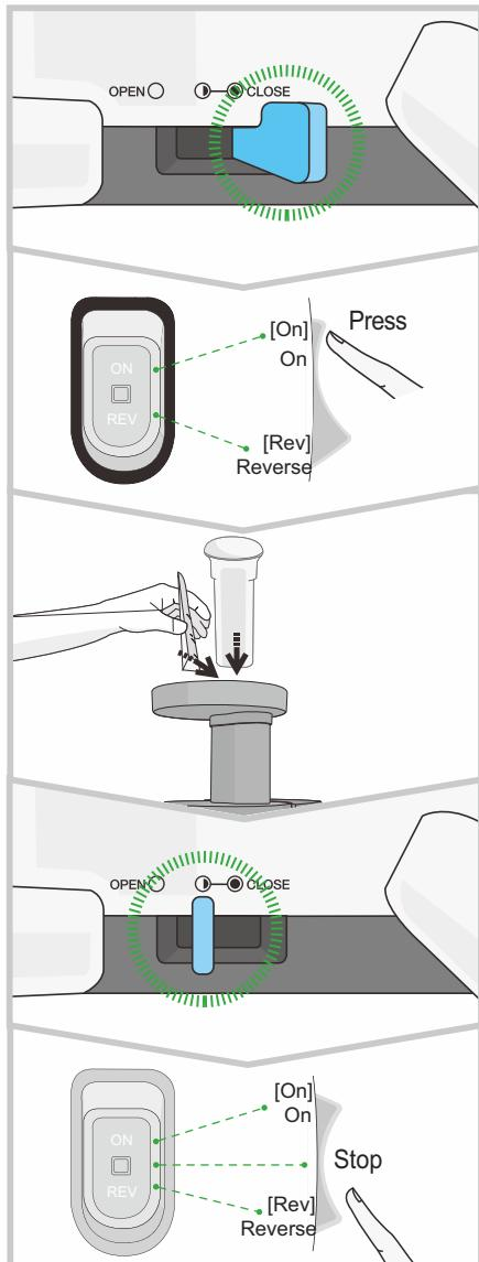
1 Place the pulp-lever in the **CLOSE** position before operating.
